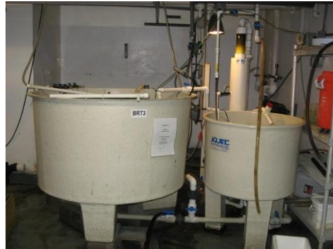
Figure 6. High density recirculating rotifer production system (1000L).
